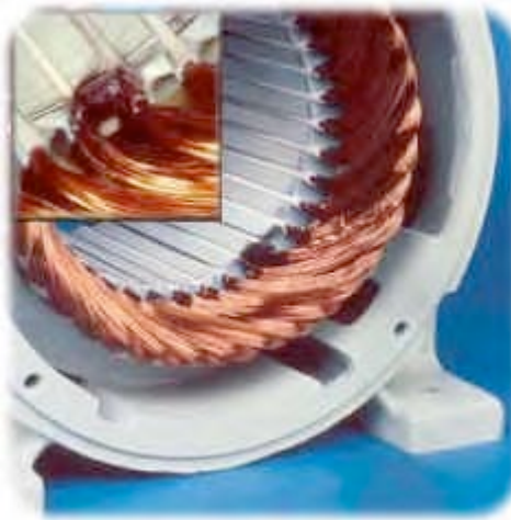
Winding Grounded at Edge of Slot
