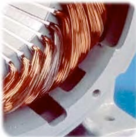
Winding with Shorted Coil
