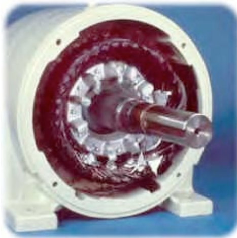
Damage Caused by Locked Rotor
