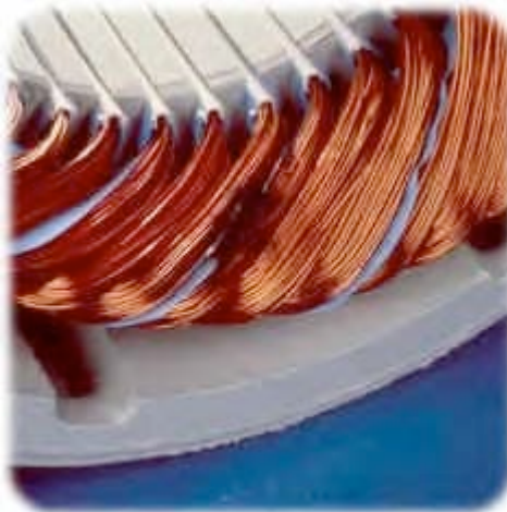
Winding Shorted Phase-To-Phase
