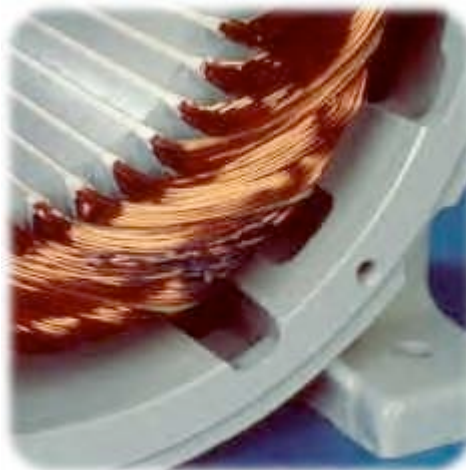
Winding Shorted Turn-To-Turn
