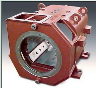
Joliet C75YZ New Drilling Frame Opposite Drive End View
